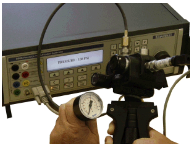
Fig 1 : Calibrating a 10Barg pressure gauge using the Druck PV411 hand pump and 0-10Barg transducer.
